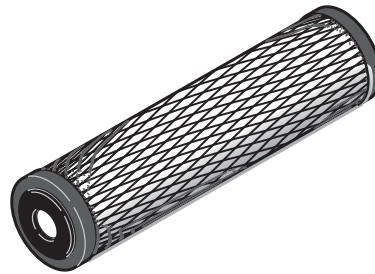
Standard Merlin Prefilter 5-micron nominal 3 NTU max turbidity 5000 gal capacity 1 ppm chlorine max at inlet
